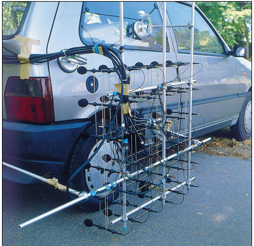
Fig.1 Microphone array positioning for tyre noise measurement on a moving vehicle
